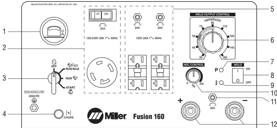
1. Engine Hour Meter/Idle Control
